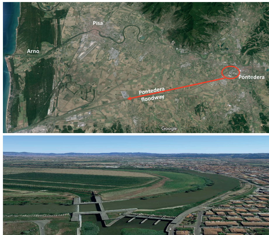
Fig. 3-1. The Pontedera floodway delivers up to 1 400 m 3 /s directly to the Tyrrhenian sea, thus mitigating the risk that the Arno may flood the city of Pisa.
